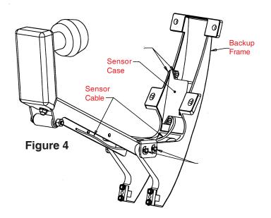
Step 3. Figure 4. To install Sensor with your RM model, remove dish from backup frame. Place Sensor inside backup frame, Figure 4. Cable must exit from bottom of Sensor. Route under pins, refer to Figure 4. Be sure case is placed so mounting screws are completely in slots. Fasten Sensor case to frame, being careful not to overtighten screws. Secure Sensor cable to coax with wire ties. Go to Step 9.
